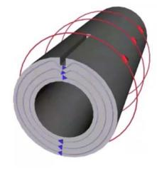
Benefit from the use of the **ec-work/** probolog<sup>™</sup> Advanced Saturated Eddy Current technology for the sensitive and fast inspection of Carbon steel and Duplex tubes in all kinds of heat exchangers, reactors or many other tube and non-tube applications.
